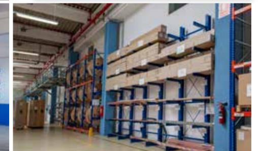
This storage system is so versatile that different component combinations can be used in various situations. The cantilever arms can be easily adjusted in height.
